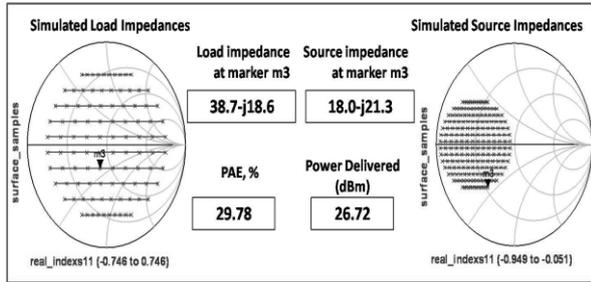
Figure 3. Simulated load and source impedance for maximum power and gain for power stage .
