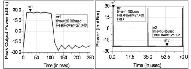
Figure 5. Simulated peak power of a single pulse (a) pulse-train (b) two stage amplifier for 8 dBm driving power.
