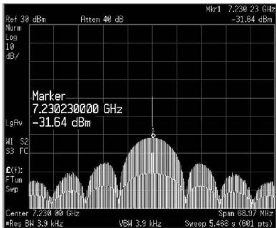
Figure 9. Line spectrum of driver stage for 8 dBm input power.
