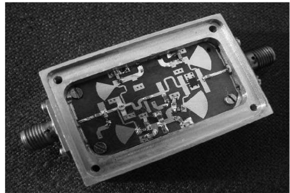
Figure 7. Prototype two stage amplifier housed in aluminum box.
