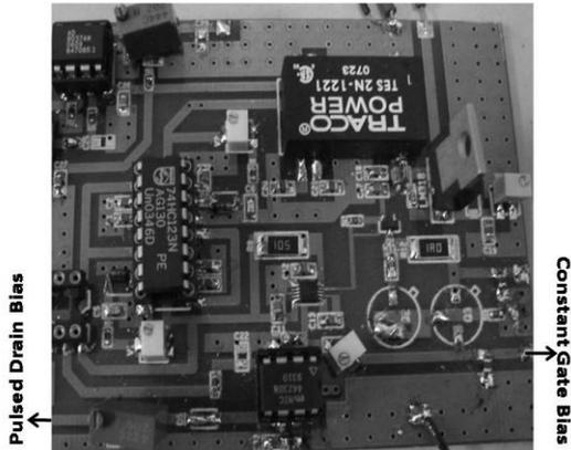
Figure 8. Pulse aggregate card.
