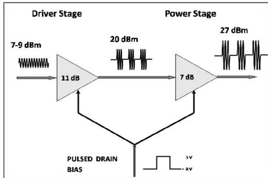
Figure 1. Energetic schematic representation of two stage pulse power amplifier.
