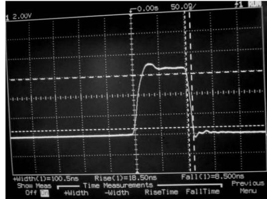
Figure 10. Modulation control pulse.
