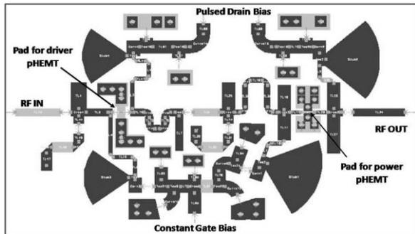
Figure 4. Layout of final two stage amplifier.
