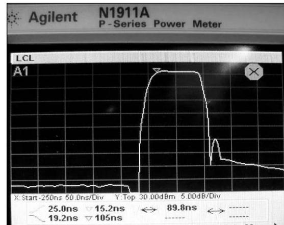
Figure 11. Measured pulse profile and rise/fall time of the prototype amplifier with peak power of 26.58 dBm.
