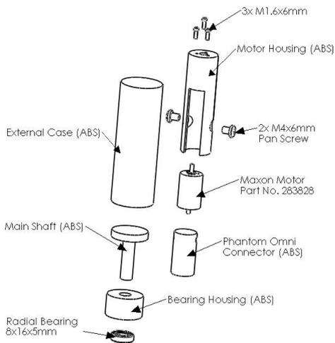
Figure 1. Exploded view of stylus and drive system
