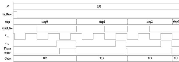
Figure 6. An example of the frequency acquisition @600MHz
