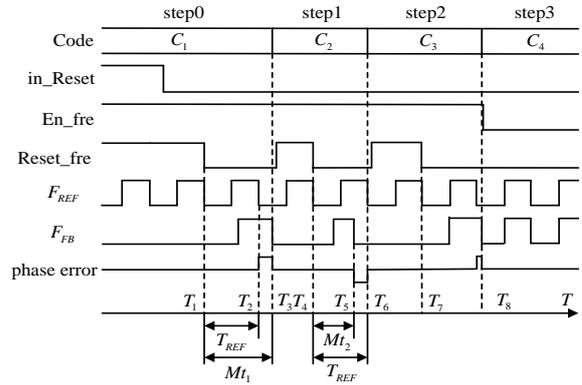
Figure 4. The waveforms of the related signals
