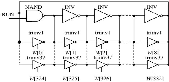
Figure 3. The structure of the DCO
