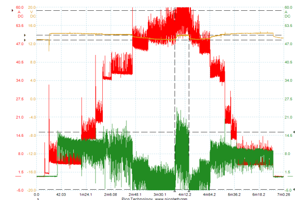
Figure 9. Car accessory current and batter voltage graphs (engine accelerating)
