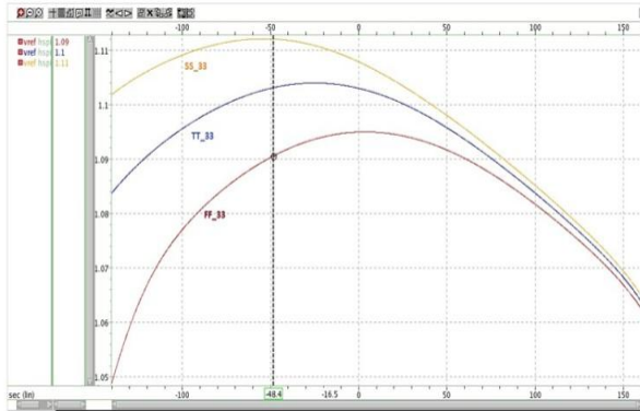
Figure 8. Bandgap temperature variation test @ TT, FF and SS corner
