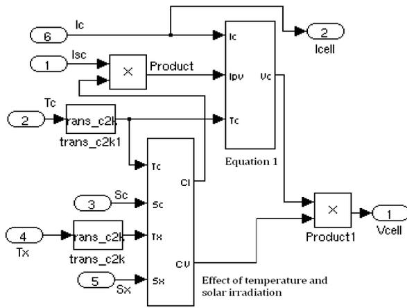
Figure 5. Functional of photovoltaic array block diagram.
