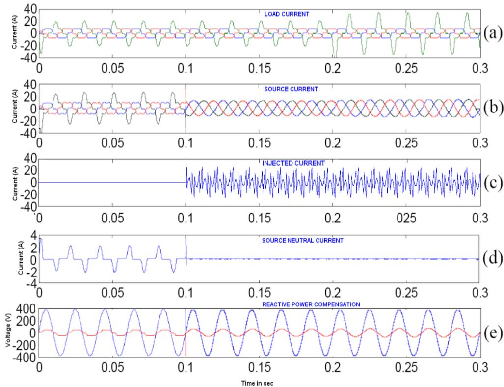
Figure 11. Load current (a), source current (b), Injected current (c), neutral current (d) and reactive power compensation (e) under dynamic load changes.
