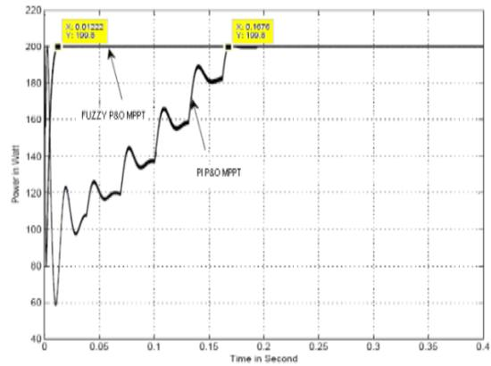
Figure 15. A single panel output by MPP tracking P&O fuzzy logic controller method
