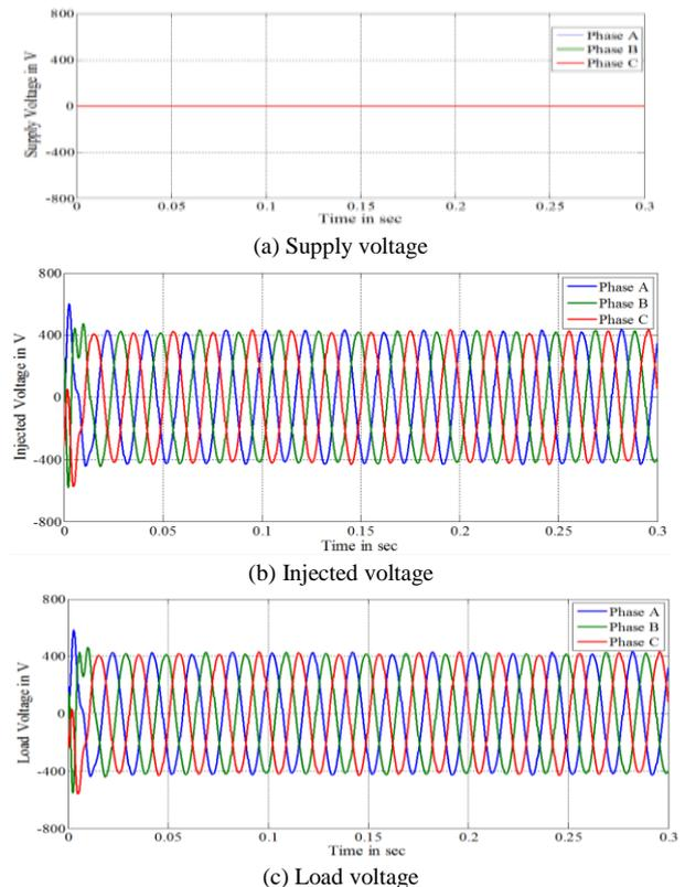
Figure 16. Supply injected and load voltage of the 3-phase PV-SAF
