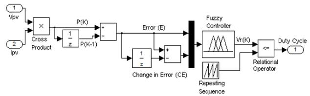
Figure 7. Control structure of fuzzy P&O MPPT
