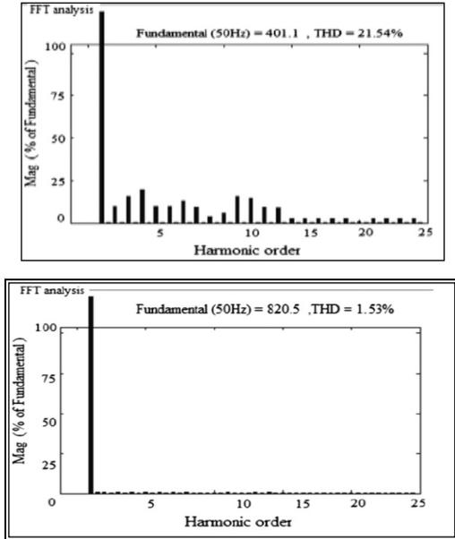
Figure 13. Phase A current THD spectrum before and after compensation
