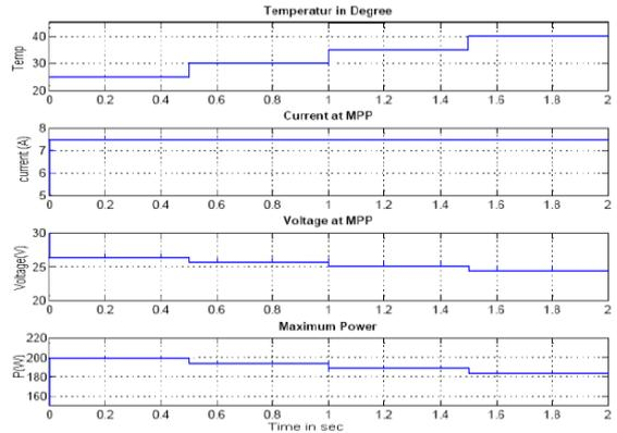
Figure 14. Simulation result of maximum current, voltage and power with Varying temperature and constant irradiation i.e. at 1000W/m<sup>2</sup> by fuzzy MPPT controller
