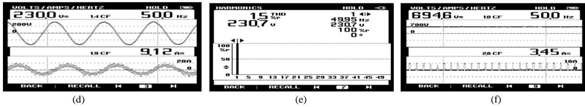
Figure 19. SAF results under Unbalanced load condition
