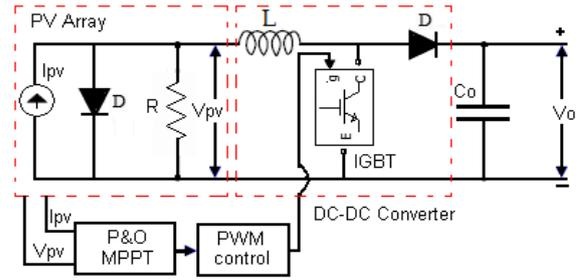
Figure 4. PV boost converter with P&O MPPT algorithm
