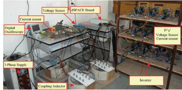
Figure 18. Overall PV-SAF Experimental Setup
