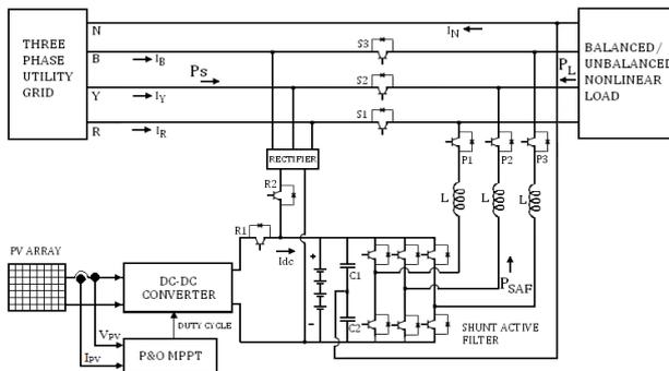
Figure 1. Block diagram of the proposed PV-SAF
