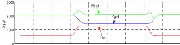
Figure 12. Source, injected and load real power under dynamic load condition.
