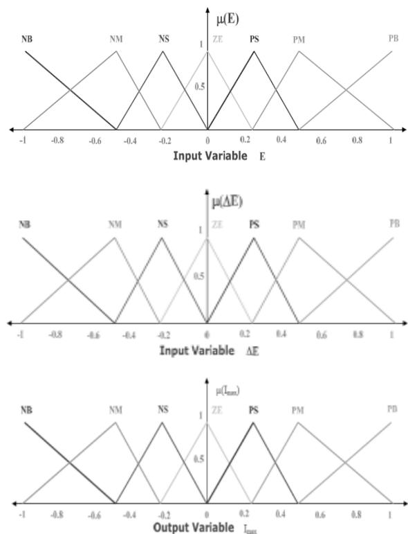
Figure 10. Membership function for variable E, CE and output
