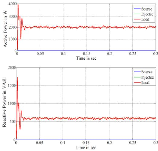
Figure 17. Active and reactive power of the PV-SAF
