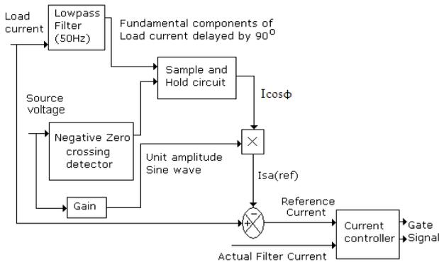
Figure 2. Block diagram implementation of IcosΦ algorithm for a phase
