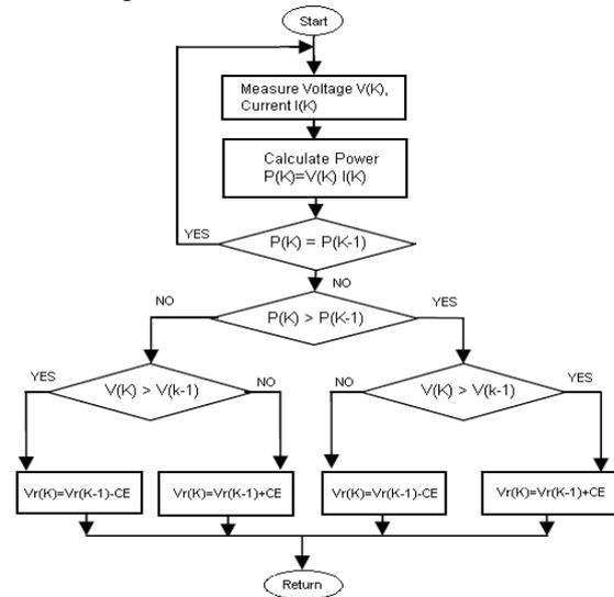
Figure 6. Flow chart of P&O MPPT algorithm
