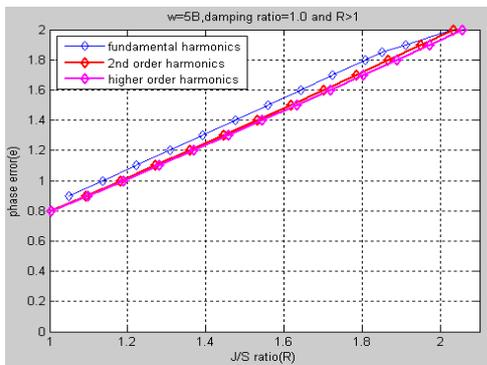
Figure 5. (c) Phase error Vs J/S ratio,  $\zeta = 1.0$ ,  $\Delta\omega = 5B$
