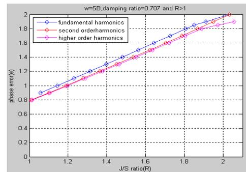
Figure 4. (c) Phase error Vs J/S ratio,  $\zeta = 0.707$ ,  $\Delta\omega = 5B$
