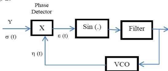
Fig. 2. A basic phase locked loop
