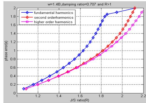
Figure 4. (a) Phase error Vs J/S ratio,  $\zeta = 0.707$ ,  $\Delta\omega = 1.4B$
