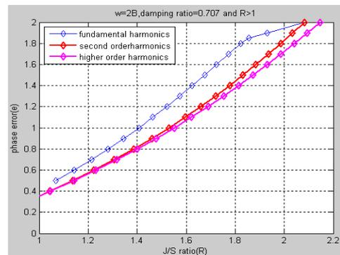
Figure 4. (b) Phase error Vs J/S ratio,  $\zeta = 0.707$ ,  $\Delta\omega = 2B$
