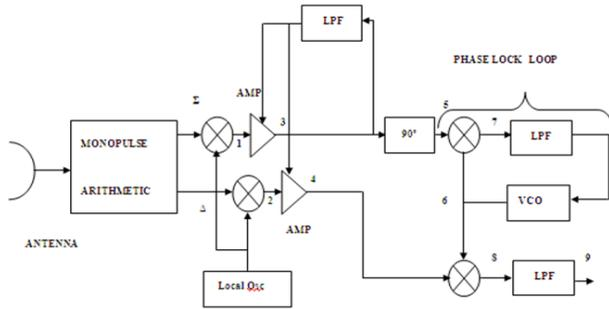
Figure 1. Monopulse receiver block diagram
