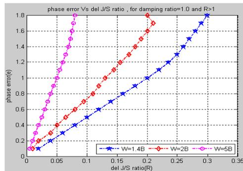
Figure 6. (b) Phase error Vs additional J/S ratio,  $\zeta = 1.0$
