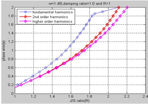
Figure 5. (a) Phase error Vs J/S ratio,  $\zeta = 1.0$ ,  $\Delta\omega = 1.4B$
