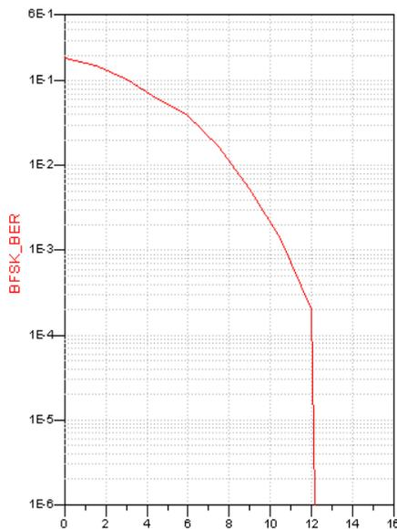
Figure 17. BER plot versus EbtoNo (dB) using the zero crossing demodulator
