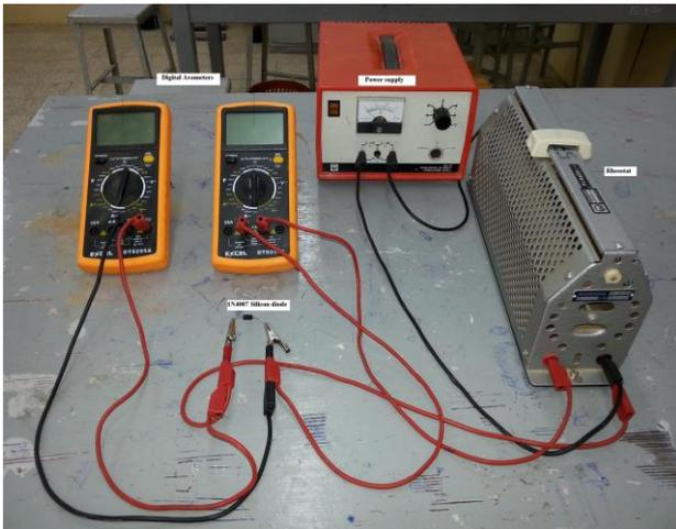
Figure 3.5. Setup for I-V measurements for pre irradiated 1N4007 silicon diode
