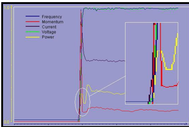
Figure 7. The without load 1500rpm frequency-moment-current-voltage-power curves of the AM
