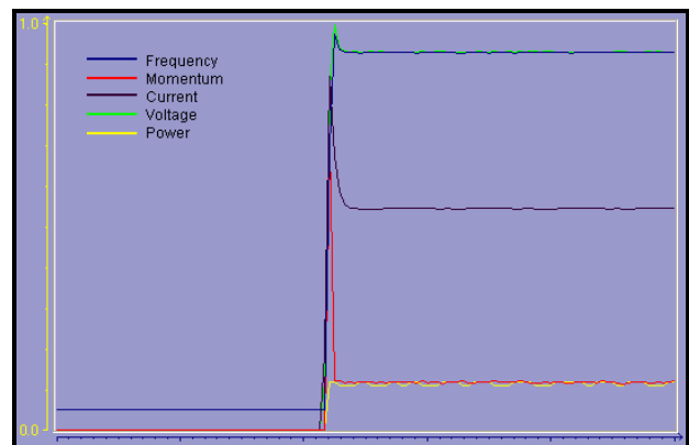
Figure 5. The without load 500rpm frequency-moment-current-voltage-power curves of the AM
