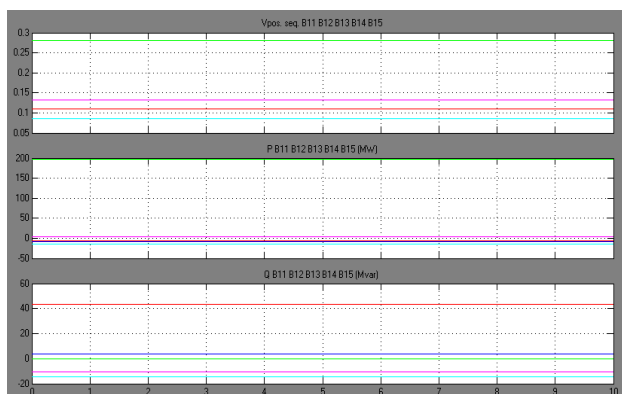
Figure 5. Voltage magnitude, real power and reactive power waveforms of bus (B11-B15) for stage I.
