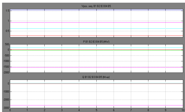
Figure 3. Voltage magnitude, real power and reactive power waveforms of bus (B1-B5) for stage I.
