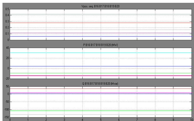
Figure 6. Voltage magnitude, real power and reactive power waveforms of bus (B16-B20) for stage I.
