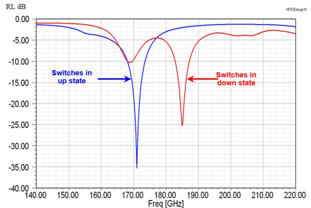
Figure 3. Simulated results of return loss antenna at different switch states
