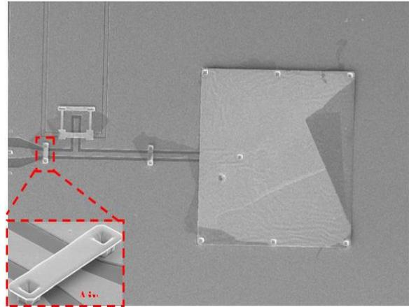
Figure 2. SIM photo of fabricated reconfigurable antenna
