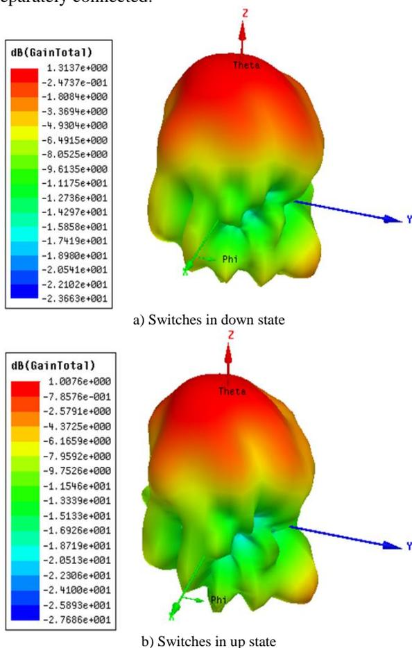
Figure 5. Simulated radiation pattern (gain dB)
