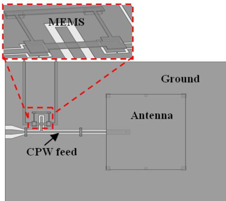
Figure 1. The configuration of rectangular elevated patch antenna design
