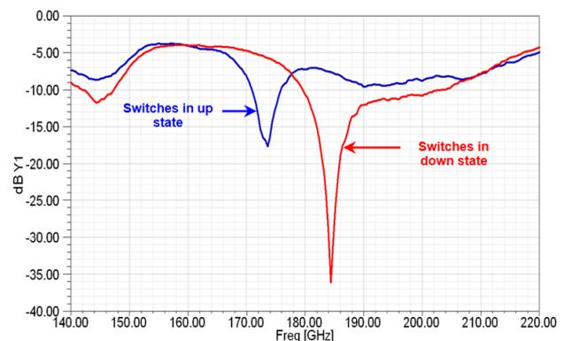
Figure 4. Measured results of return loss antenna
