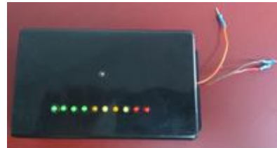
Figure 8. The notepad of 10-steps LED light bar for sEMG signal quality monitoring.
