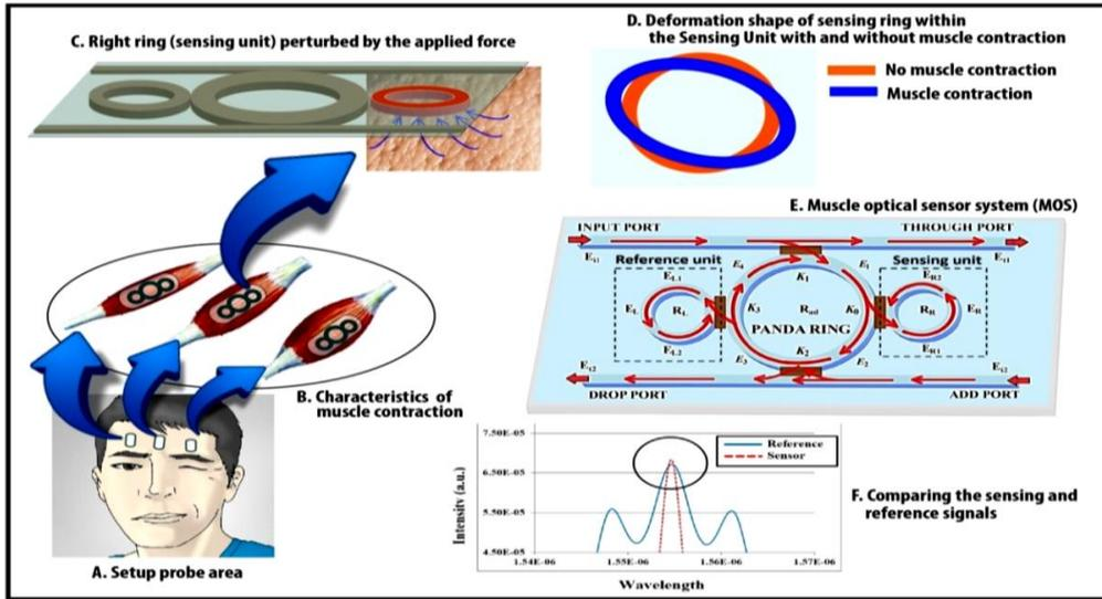
Figure 2. Schematic diagram of principles and the experimental concepts.
