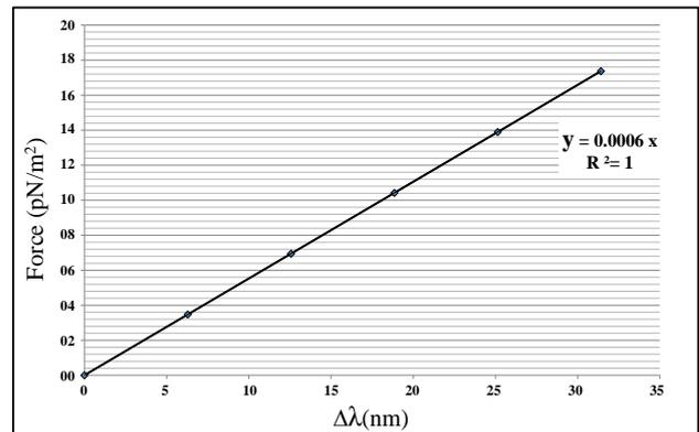
Figure 4. Graph of the linear relationship between force and the wavelength shift ( $\Delta\lambda$ )
