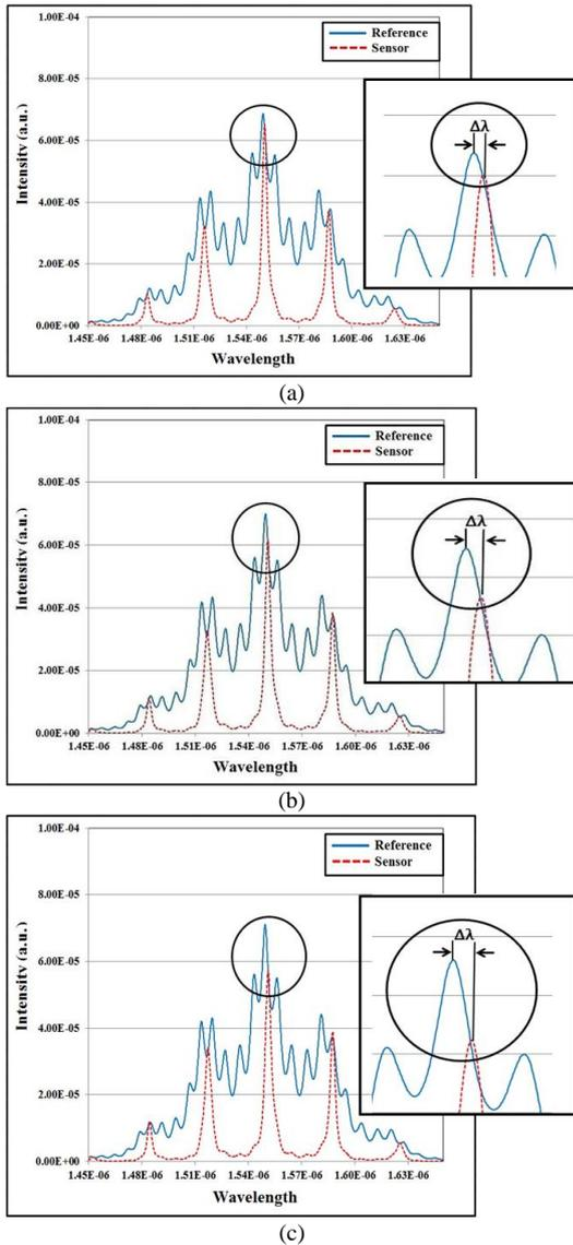
Figure 3. Shows the relationship between intensity and wavelength of sensing ( $E_R$ ) and reference signals ( $E_L$ ), with the radius  $R_L$  (blue line) and  $R_R$  (red line) is varying form 3.249-3.254  $\mu\text{m}$ , (a)  $R_R = 3.251 \mu\text{m}$ , (b)  $R_R = 3.252 \mu\text{m}$  and (c)  $R_R = 3.253 \mu\text{m}$
