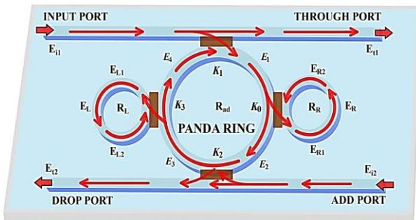
Figure 1. Schematic diagram of the MOS using PANDA ring resonator and deformation shape of sensing ring within the sensing unit with and without external force, where  $R_s$  is ring radii,  $\kappa_s$  is coupling constant, and  $E_s$  is optical fields.
