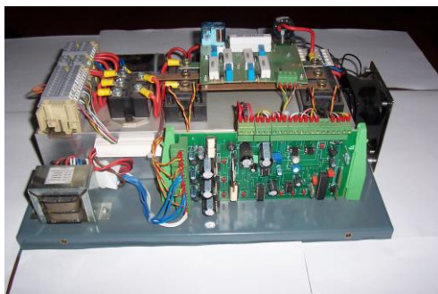
Figure 4. Implementation of the welding machine
