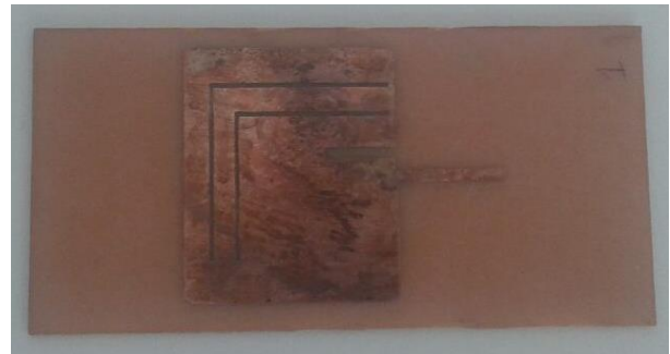
Figure 6. Fabricated circuit I with L-shaped slots.
