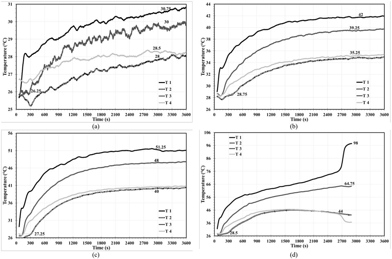
Figure 4. Results of the loop of a 100 cm width with the expansion tank close to the cooler arm at heater voltage (a) 28 volts (b) 56 volts (c) 84 volts (d) 112 volts.
