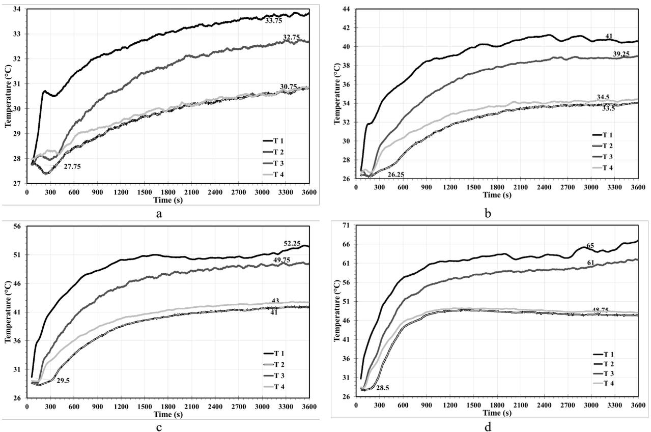
Figure 5. Results of the loop of a 100 cm width with the expansion tank close to the heater arm at heater voltage (a) 28 volts (b) 56 volts (c) 84 volts (d) 112 volts.
