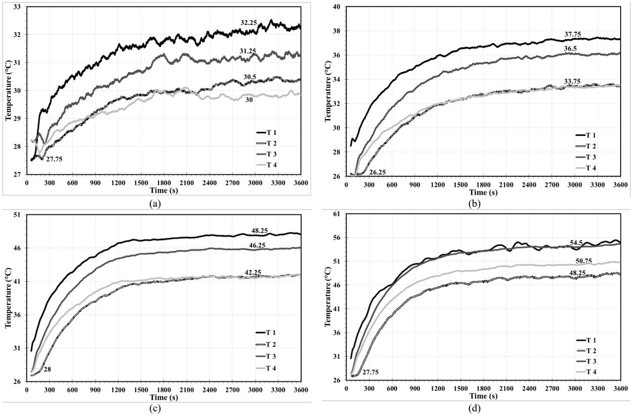
Figure 3. Results of the loop of a 50 cm width at heater voltage (a) 28 volts (b) 56 volts (c) 84 volts (d) 112 volts.
