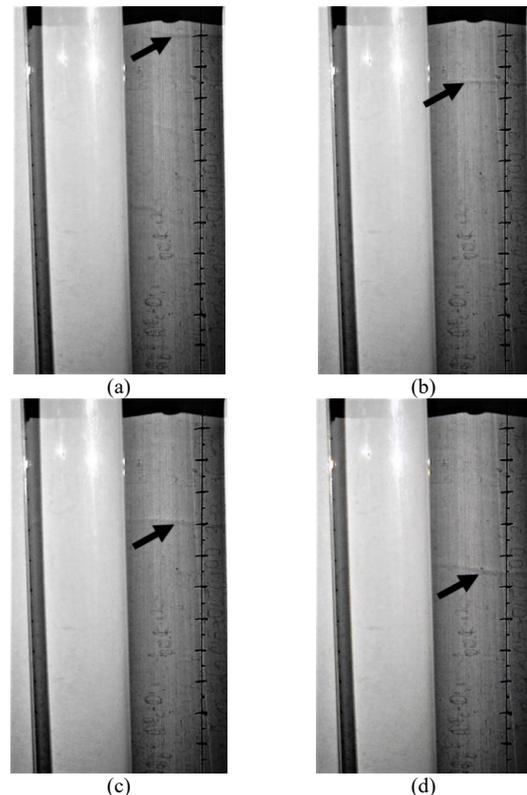
Figure 6. Visual observations of a natural circulation loop of 50 cm width at (a) 56,68 s, (b) 57,01 s, (c) 57,34 s, and (d) 57,68 s.
