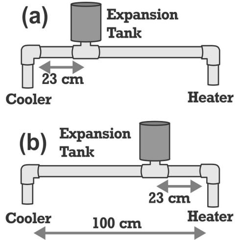
Figure 2. The loop of a 100 cm width with (a) the expansion tank close to the cooler arm and (b) the expansion tank close to the heater arm.
