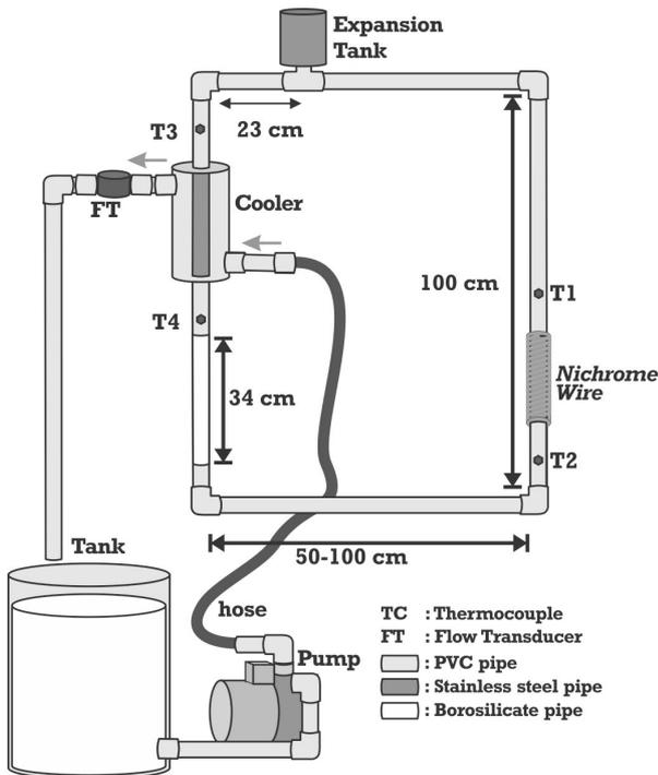
Figure 1. Sketch of single-phase natural circulation loops experiment apparatus.
