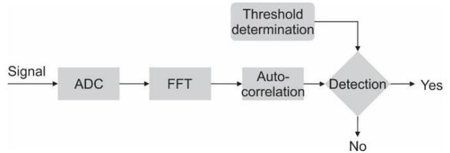
Figure 2. ED in frequency domain block diagram.
