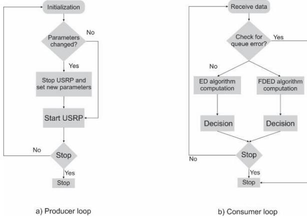
Figure 9. Producer and consumer loop block diagrams.
