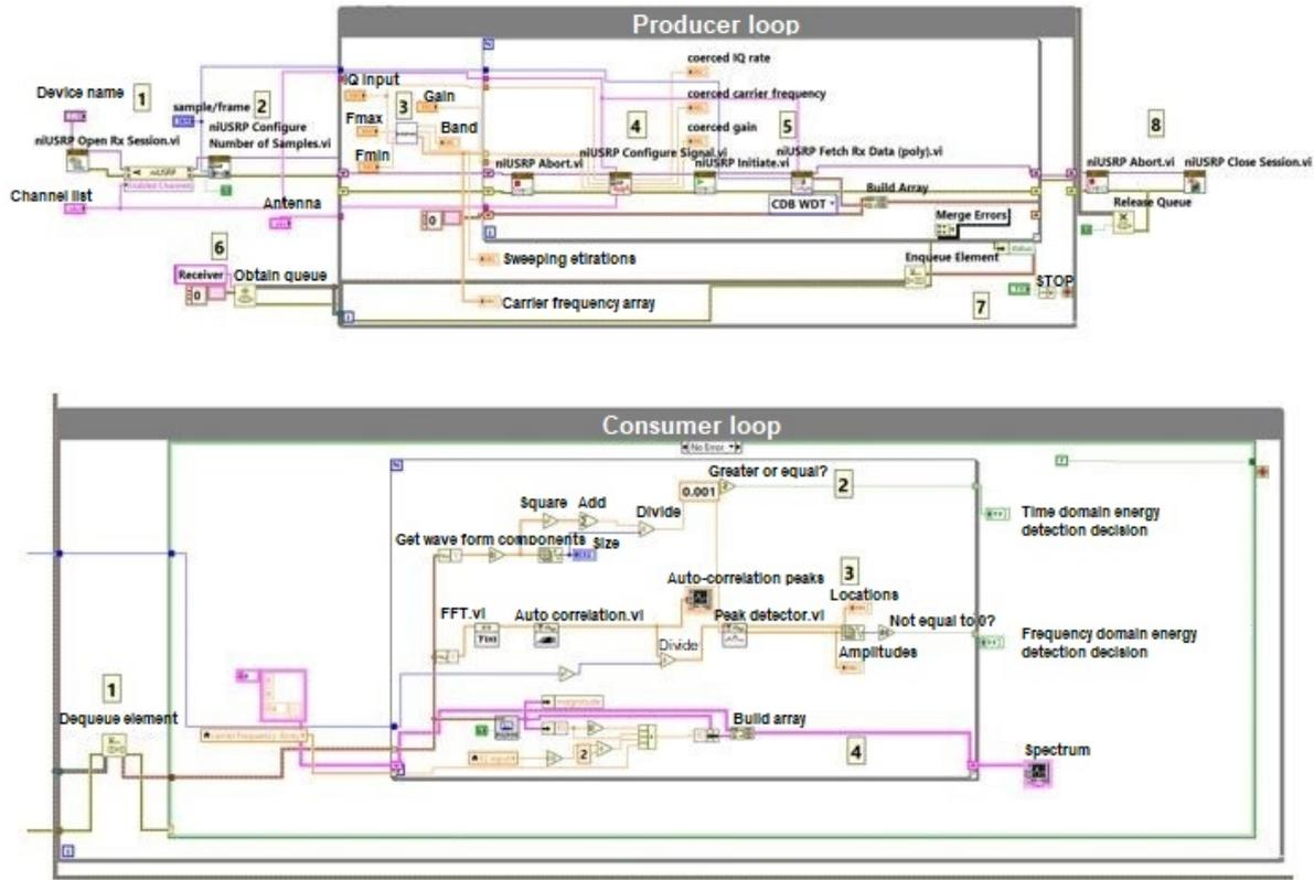
Figure 13. Receiver block diagram producer and consumer loop.
