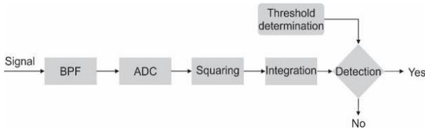
Figure 1. ED block diagram.
