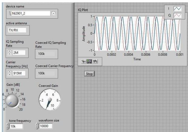
Figure 10. Transmitter front panel.
