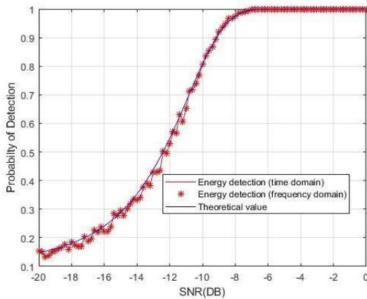
Figure 5. ROC of energy detection analytical.
