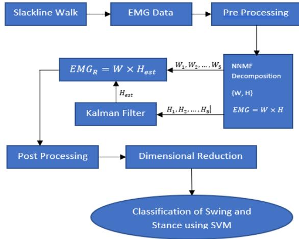
Figure 6. Schematic layout of pattern classification process using the reconstructed EMG signal.
