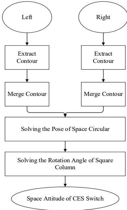
Figure 2. General process of CES switch positioning method.
