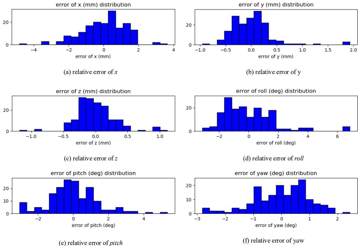
Figure 6. Distribution of relative positioning error of circular handcart.
