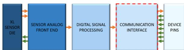
Figure 3. Simplified diagram of the accelerometer.
