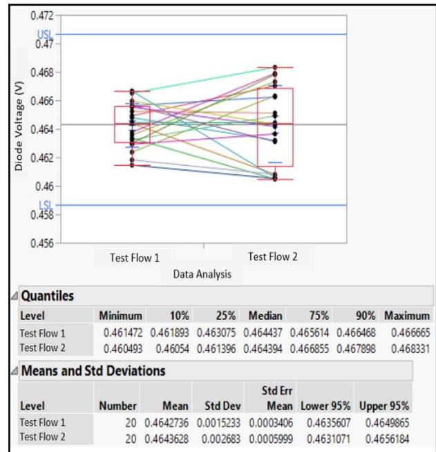
Figure 13. Serial number match plot of two test flows with different test time.
