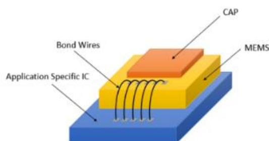
Figure 1. MEMS chip scale package.
