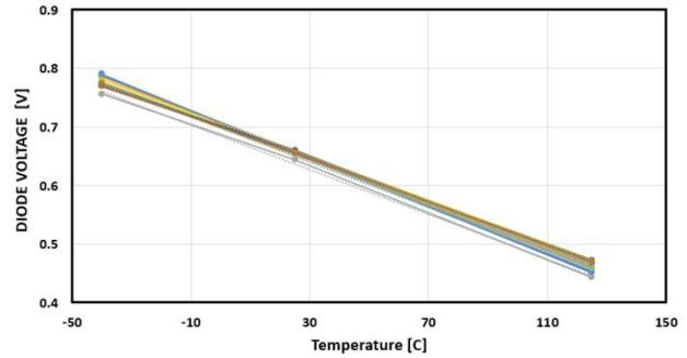
Figure 7. Plotted bench reference data (diode voltage vs. TEMPERATURE).
