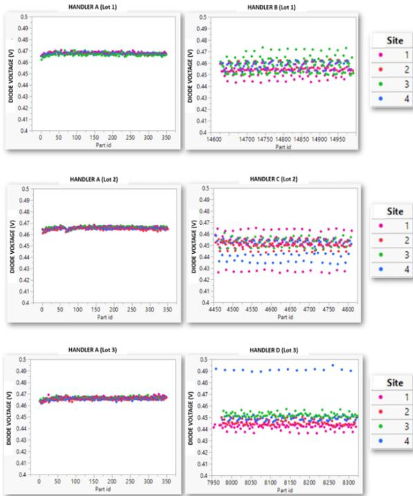
Figure 14. Plot distribution of the correlation units of the 3 lots in diode voltage parameter on the newly calibrated handler vs. other handlers.
