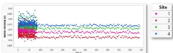
Figure 2. Sample data with observable shift of temperature sensitive parameter.
