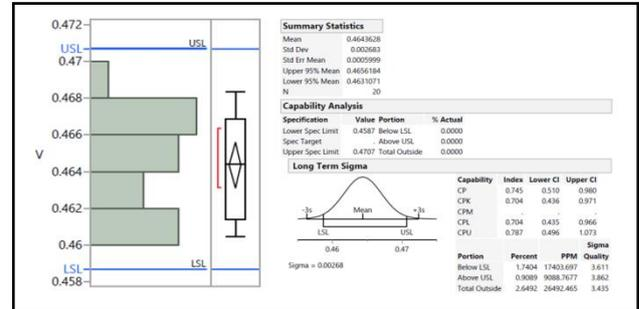
Figure 12. Golden units histogram on calibrated handler.
