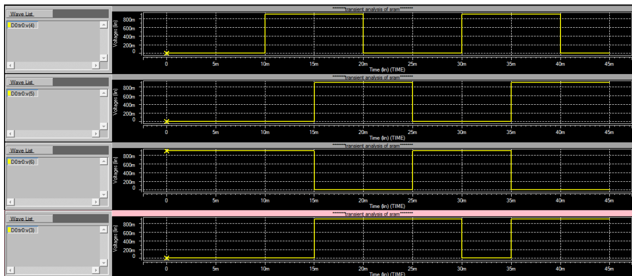
Figure 7. Simulation waveform for 6-T SRAM cell in 32nm CMOS technology
