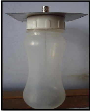
Figure 2. The typical fabricated monopole antenna in testing jar.
