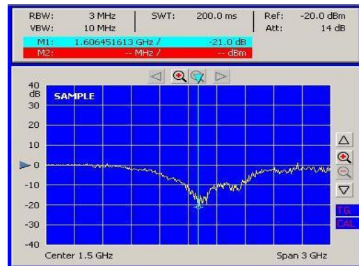
Figure 5. Resonant frequency of liquid liquid yagi-uda antenna at specified salinity (0.5 M).
