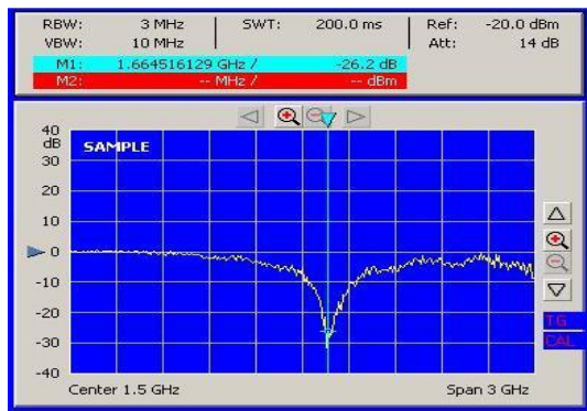
Figure 7. Resonant frequency of liquid liquid yagi-uda antenna at specified salinity (1.5 M)
