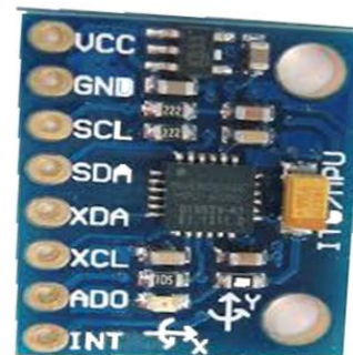
Figure 3. 6-Axis motion tracking device (MPU 6050)
