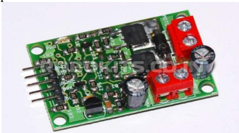
Figure 5. H-Bridge driver circuit
