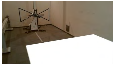
Figure 4. Background noise measurement scenery of in Anechoic Chamber (without EUT and DC power source line).
