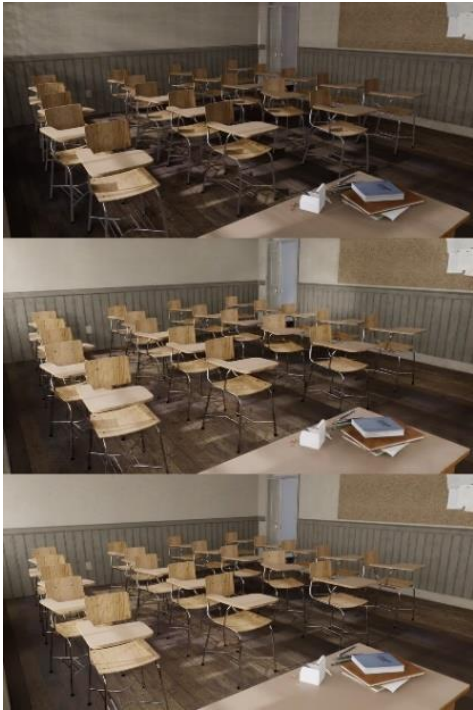
Figure 6. Blender classroom scene: Top: Rasterisation, Middle: GAN, Bottom: Raytraced.
